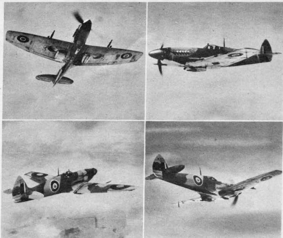
FLYING PHOTOGRAPHS OF SPITFIRE XII SHOW ITS CLIPPED WING, POINTED RUDDER AND LONG NOSE
